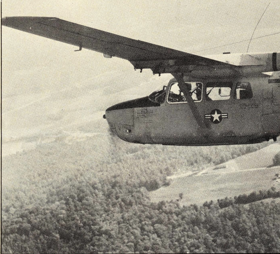
The modest variety of stores and/or armament which an O-2 might go out with can be listed on the side panel just ahead of the forward lower window.
